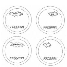
After correct selection of the day option, the ST620RF display will change to the next programming screen. These screens allow you to set the required time and temperature settings to provide optimum control for your heating system.
